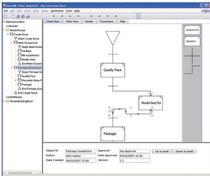
Using xfy for Batch Process Definition, R&D engineers can visually manipulate and edit an S88-based flow chart to assemble master recipes based on normalized recipe and procedural definitions. The result is a consistent recipe definition, enabling error-free technology transfer and eliminating the need for re-keying information between phases. This accelerates time to market, reduces operational costs and dramatically reduces the risk, waste and poor quality associated with inaccurate recipes.
